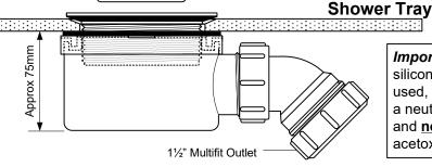
Important: If a silicone sealant is used, it should be a neutral sealant and not an acetoxy sealant.
